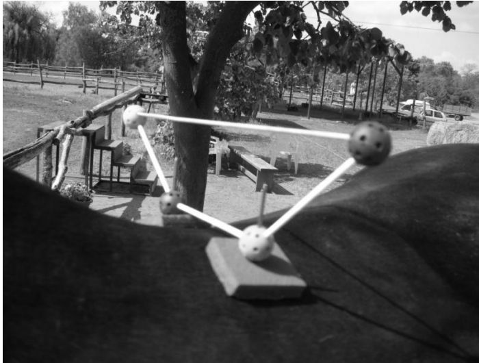
Figure 2. The trapezoid frame markers representing the human pelvis model of the rider
